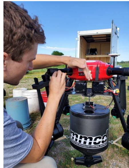
Figure 7.2 Adjusting the voltage to the treatment hopper.
